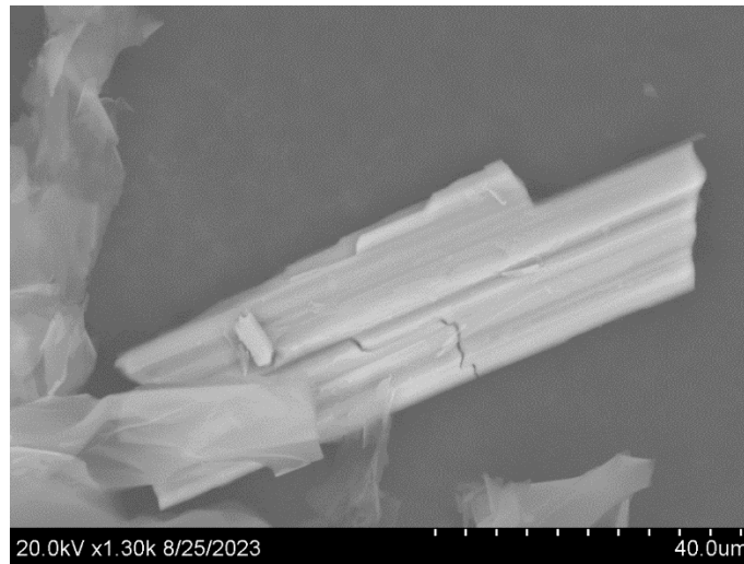
Figure 7- Reference images of asbestos seen on SEM.
